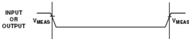
Figure 7: Voltage Reference Levels for AC Measurements (Except Output Enable/Disable)
